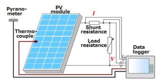
Fig. 3 Measurement system for PV module
