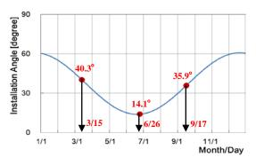
Fig. 6 Optimum installation angle (theoretical data and date of experiments)
