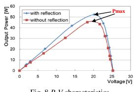
Fig. 8 *P*-*V* characteristics (examination of sunlight reflection)
