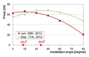
Fig. 5 Pmax when installation angle changes (experiments in June and September)
